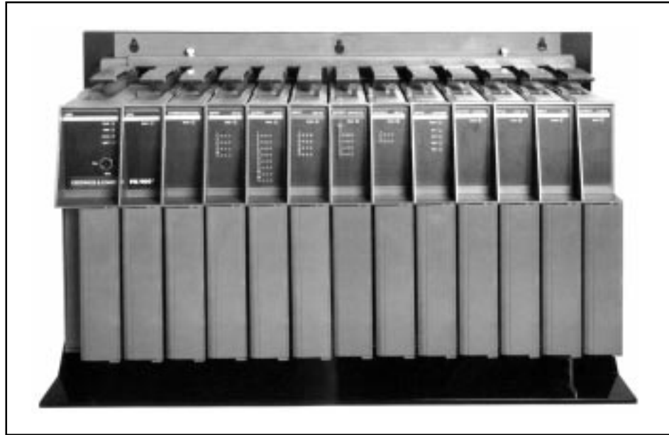
Figure 21-7. Giddings & Lewis's area C PIC900 with up to 3168 I/O and motion I/O, IEC programming, and floating-point math capabilities.
