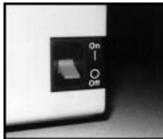
Figure 2-3. The binary numbers, 1 and 0, on a computer's power switch represent ON and OFF, respectively.
